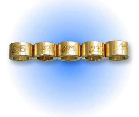
The PT Spacer Kit gives you five different brass spacers all legibly numbered so you can adjust the spacing of the power tube o-ring. If your marker has bolt stick use a longer one, if it leaks down the barrel use a shorter one. Find one that works and stick with it! Quality machined brass to AGD standards. PT Spacer Kit comes with an extra power tube o-ring not shown.
