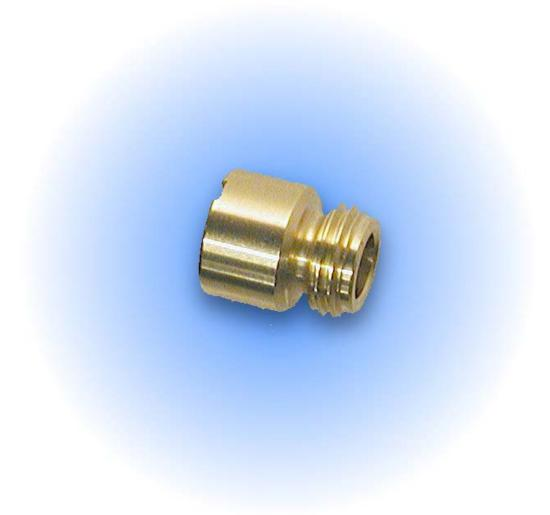
This item screws into the end of the Power Tube and is a precision part. It releases the air blast behind the ball in a controlled manner so the air hits the ball with low pressure to gently accelerate it out the barrel. Use a coin to tighten it up.
