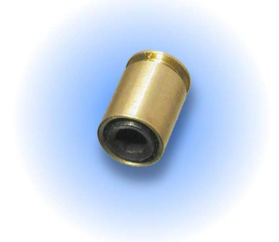
The Regulator Piston comes as an assembly. DO NOT take this apart. It has a built in blow off valve that will leak air if your marker becomes over pressurized. The blow off resets once your pressure goes back to normal. This safety feature is found exclusively in AGD markers. Replace the entire assembly if your marker is shooting at normal speeds and it still leaks out the back.
