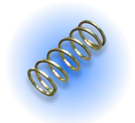
The Bolt Spring fits all AGD markers regardless of age or type. They are made from very special square wire so they don't fold inside themselves when collapsed. Replace your old springs when they sag below the front of the bolt. Special honed bolt springs come with Superbolts to prevent premature wear. One spring also comes in the Parts Kit. If you need any o-rings the kit is a good value.
